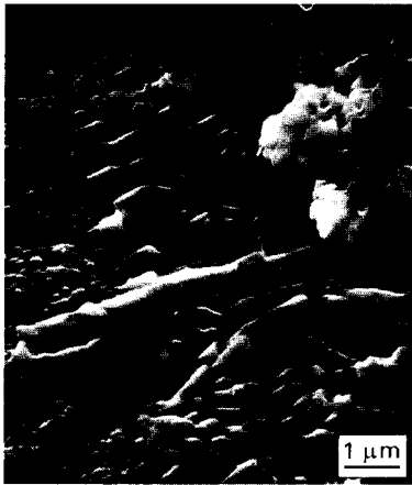
Figure 11 The top view of the etched alumina/braze interface, with alumina (grainy surface) underneath the braze. The alumina/braze reaction product remained on the alumina after etching.
